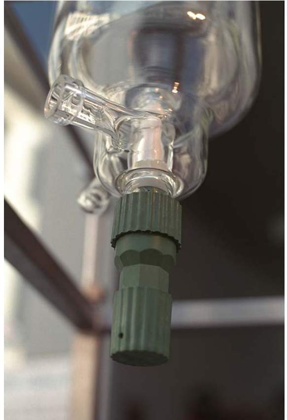
HWS-Outletvalve model „T“ with heating mantle
